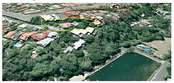
**Figure 3.18** Low angle, north-west facing 3-D image of the quarry site showing the probable edges of the quarry (marked in red) and the possible lower quarry site where the railway terminated (marked in yellow) (source: Google Earth).
